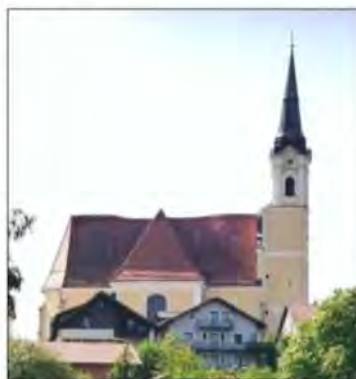
Figure 7: In 1972, the Catholic church in Untergriesbach, Bavaria, was fumigated with Zyklon B. Subsequently the entire plaster turned patchy blue (Konrad Lackerbeck; Wikipedia commons).
